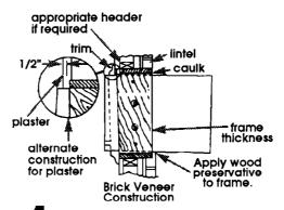
When using a wood, metal or plastic molding, the finish frame should line up with inside wall. If the plastered wall is to be flush with the cabinet and no molding is used, the finish frame must be set 1/2 inch into the wall.
