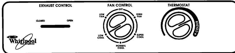
1. Set **EXHAUST CONTROL** to **CLOSED** for maximum cooling performance.
