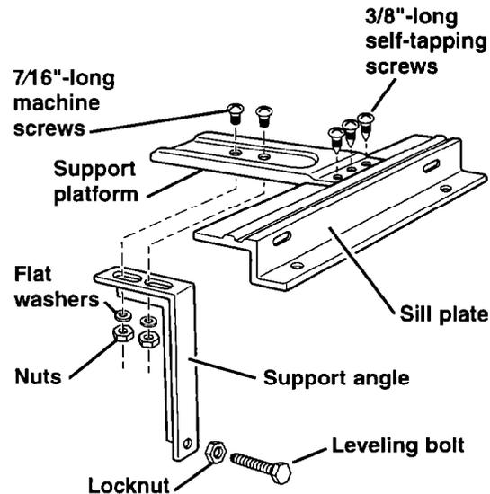
6. Place the support platform assembly against the lower window track and firmly against the vertical edge of the window frame.
