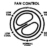
Do not try to operate your air conditioner on SUPER COOL, NORMAL COOL or LOW COOL when outside thermostat is below 65°F. The inside evaporator coil will freeze up and the air conditioner will not operate properly.
