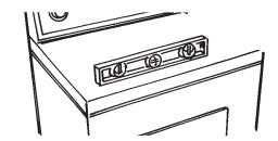
Check levelness of dryer by placing a level on top of dryer, first side to side, then front to back. If dryer is not level, adjust dryer legs up or down.
