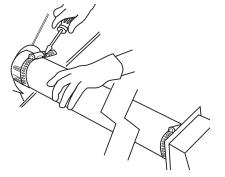
Connect vent to dryer outlet using a 4" clamp. If connecting to existing vent, make sure the vent is clean. The vent must fit over the dryer outlet and inside the exhaust hood.
