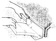
To remove the screen, open the lid and pull the screen straight out. Roll the lint off the screen with your fingers. **DO NOT rinse the screen or wash it.** Wet lint is hard to remove. When replacing the screen, push it firmly into place. Close the lid.
