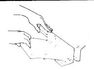
To remove the screen, open the lid and pull the screen straight out. Roll the lint off the screen with your fingers.
