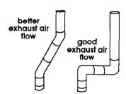
Metal flexible duct must be fully extended and supported when the dryer is in its final position. DO NOT KINK OR CRUSH THE DUCT. The metal flexible duct must be completely open to allow adequate exhaust air to flow.
