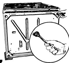
Start to screw the legs into the holes by hand. Use a 1" (2.5 cm) socket wrench or other type wrench to finish turning the legs until you reach the diamond marking.
