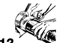
Connect exhaust duct to exhaust hood and dryer. (See Exhaust requirements, Panel B.)
