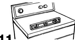
■ Check levelness of dryer by placing level on top of the dryer, first side to side, then front to back. If dryer is not level, adjust the legs of the dryer up or down. Dryer must be level to prevent noise and poor drying performance.
