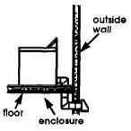
Mobile home exhaust requirements: The dryer must have an outside exhaust. If the dryer is exhausted through the floor and the area under the mobile home is enclosed. the exhaust system must terminate outside the enclosed area. Extension beyond the enclosure will prevent lint and moisture buildup under the mobile home.
