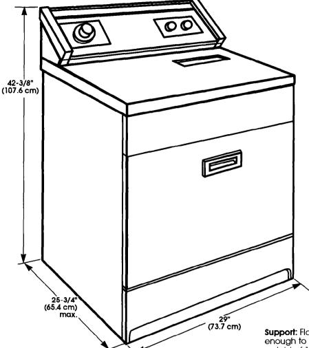
**Level floor:** 1-inch (2.5 cm) maximum slope under <u>entire</u> dryer.
