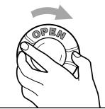
cover from the back wall of the dryer by turning the cover clockwise. **3.** Remove the light bulb by turning it counterclockwise.
