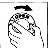
cover from the back wall of the dryer by turning the cover clockwise.
