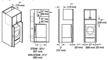
\*Required spacing \*\*For side or bottom venting, 0" (0 mm) spacing is allowed.
