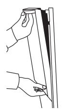
2 Completely open oven door. Insert small end of a door removal pin into each door hinge. Grasp door handle from the bottom and gently close door as far as it will shut. Lift slightly and grasp bottom of door with other hand. Pull door out at bottom to remove. Set door aside on protected surface.
