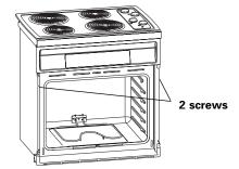
6 Important: Securely fasten range to cabinet using the two screws provided. Insert the screws through holes in mounting rails. Do Not overtighten screws.
