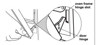
Replace the oven door by inserting ends of hinges into hinge slots in range frame. Push behind each hinge so that hinges are pushed into range frame as far as they will go. Open door and remove both door removal pins. Close and open door to check that door closes and opens completely. If door does not close or open completely, you have not pushed hinges completely into frame. Repeat door removal step and reinsert door into hinge slots again.
