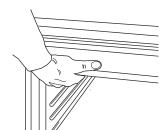
Lift range into cabinet cutout using the oven opening as an area to grip. Be careful not to damage countertop.
