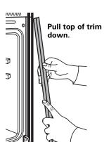
Remove trim screws attaching right and left side trim to range. Grasp the bottom end of trim and pull away from range. Slide top end of trim downward to remove trim from range. Take care not to scratch other surfaces with ends of trim. Set trim and screws aside on protected surface.
