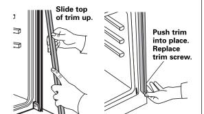
Slide top end of each trim upward onto range side rails. Push each trim into place at bottom of trim. Use screws to attach each trim to range. Take care not to scratch other surfaces with ends of trim.
