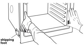
To avoid damaging the countertop, lift range slightly while pushing against seal area of front frame. Push range into cabinet cutout until shipping feet almost contact cabinet. Use a Phillips screwdriver to remove screws attaching shipping feet. Remove and discard shipping feet.
