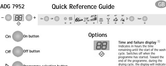
drying cycle, the display will indicate the time remaining in minutes. "F..." Identification of faults for service technician
