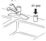
Make sure to use an air gap if the drain hose is connected to house plumbing lower than 20" (50.8 cm) above subfloor or
