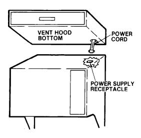
Reach through hole in bottom of vent hood, pull out power cord until all slack is removed.
