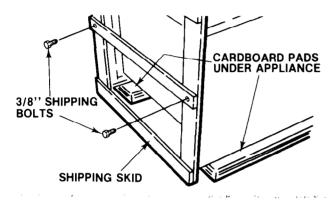
Remove the 4 cardboard pads from shipping box. Place them on floor as shown to protect appliance's finish. Rest appliance (on its back) on pads.
