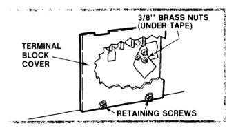
Terminal block cover is located on back of the appliance near the bottom.
