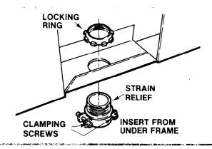
Disconnect clamping ring from strain relief. Push relief (from bottom) through hole beneath terminal block. Tighten clamping ring (from above) onto strain relief threads.
