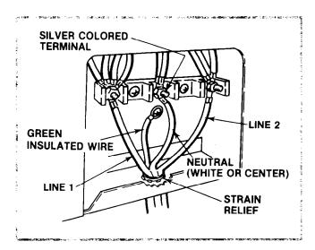
Use this wiring method for mobile homes and whenever a 4-wire installation is required.
