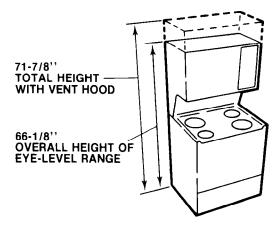
Install vent hood **BEFORE** making final electrical connection,
