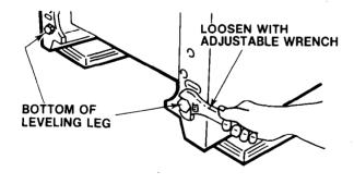
Once skid is removed, 4 leveling legs are exposed at bottom of frame.
