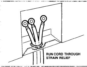
Run cord or cable through strain relief.
