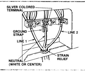
Use this wiring method ONLY if local codes permit connecting frame grounding conductor to neutral wire of power cord.
