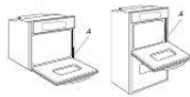
Single Oven A: Mounting rail on cabinet plate Double Oven A: Mounting rail on cabinet plate
