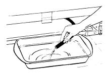
Unclip hose and allow defrost water to drain through the hose into a flat pan. After defrosting and cleaning, hook drain hose in place and replace the base grille and drain cap.
