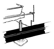
2. Keep it level – Level your freezer by adjusting the two leveling legs at the front corners. (Adjust door-hinge side first.) Turn left to raise the corner; right to lower it. When freezer is sitting level, the freezer door (when opened) will stay at any open position. After the freezer has been filled, recheck to see if it is sitting level.
