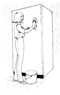
Wash outside of freezer with warm water, using a mild soap or mild detergent. Rinse and dry. Do not use an abrasive or harsh cleanser. Waxing is not recommended.
