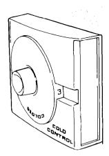
Set cold control – The cold control is located inside your freezer on the right wall. To start, turn cold control to middle of dial. This position will maintain zero zone temperatures under normal operating conditions. Turn the cold control to a higher number for colder temperatures or a lower number for less cold temperatures.
