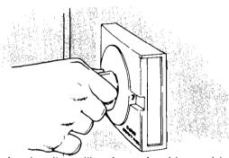
Before loading with unfrozen food, turn cold control to coldest position (highest number) and let freezer operate for several hours. This will speed up the rate of freezing. Lay packages to be frozen in a single layer so each rests on the freezing surface of a shelf. Allow space between packages for cold air to circulate.
