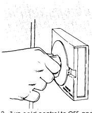
Turn cold control to OFF, and disconnect service cord from wall outlet.
