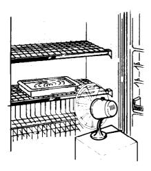
4. Place pans of hot water inside freezer to hasten melting of frost. Leave door open. As ice softens and melts, it can be removed in large pieces. Direct air from an electric fan into the freezer to speed defrosting.
