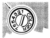
Set cold control – Insert a coin in the slot of the control to turn it. To start, turn cold control to Number 3. This position will maintain zero zone temperatures under normal operating conditions. Turn the cold control to a higher number for colder temperatures or a lower number for less cold temperatures.
