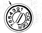
Set cold control – Insert a coin in the slot of the control to turn it. To start, turn cold control to Number 3. This position will maintain zero zone temperatures under normal operating conditions. Turn the cold control to a higher number for colder temperatures or a lower number for less cold temperatures.
