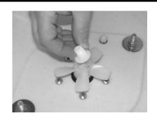
Step 3: Remove the impeller knob by turning counter clockwise.
