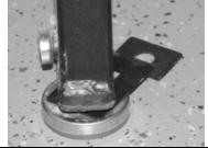
Step 3: Mark spots to be drilled. Bracket has ½" hole. If mounting to floor, use (2) 3/8" floor lag bolts with washer – not provided.
