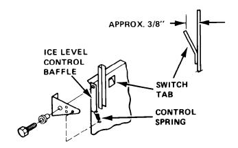
NOTE: Baffle must swing freely without binding.
