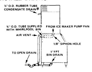
**NOTE:** The  $\frac{1}{6}$ " dia. siphon break hole must be in the vertical leg of white vinyl tubing.
