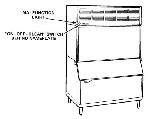
Electrical Supply 115-208/230 V. 3-Wire 60 Hz—1 Ph.
