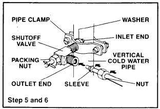
6. Slip compression nut and compression sleeve on copper tubing as shown in diagram. Insert end of tubing into outlet end squarely as far as it will go. Screw compression nut to outlet end with adjustable wrench. Do not overtighten. Turn ON main water supply and flush out tubing until water is clear. Turn
