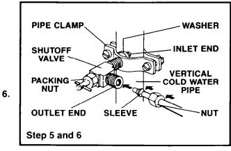
Slip compression nut and compression sleeve on copper tubing as shown in diagram. Insert end of tubing into outlet end squarely as far as it will go. Screw compression nut to outlet end with adjustable wrench. Do not overtighten. Turn ON main water supply and flush out tubing until water is clear. Turn OFF shutoff valve on the water pipe. You are now ready to connect other end of 1/4-inch copper tubing to inlet tube or water valve on back of refrigerator.
