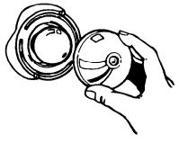
Replace the bulb cover and snap the wire holder into place. Plug in appliance or reconnect at the main power supply.
