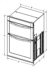
30" (76.2 cm) models **30°** (76.2 cm) models A. 42% (\* (108.0 cm) overall height B. 28½ (\* (72.3 cm) recessed width C. 41\* (104.1 cm) recessed height D. 23¼ (\* (59.1 cm) max. recessed depth E. 30\* (76.2 cm) overall width
