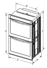
27" (68.6 cm) models 27" (68.6 cm) models A. 51 ‰ (13.0 cm) max. overall height B. 25 ‰ (64.6 cm) max. recessed width C. 48 ‰ (124.0 cm) recessed height D. 23 ‰ (59.1 cm) max. recessed depth E. 27" (68.6 cm) overall width
