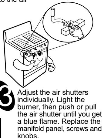
NOTE: Because of different altitudes above sea level and variations in the supply of gas, you may need to adjust the main air intake to the burners. This will result in a better air-gas mixture and thus a better operation.
