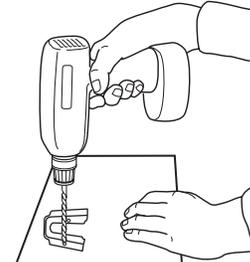
To mount anti-tip bracket to concrete or ceramic floor, use a ⅜" (0.48 cm) masonry drill bit to drill 2 holes at the positions marked on the bracket template. Remove template from floor.
