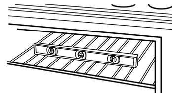
3. If range is not level, pull range forward until rear leveling leg is removed from the anti-tip bracket. Use 3/8" drive ratchet and wrench or pliers to adjust leveling legs up or down until range is level.
