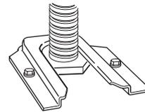
12. If installing the range in a mobile home, you must secure the range to the floor. Any method of securing the range is adequate as long as it conforms to the standards in the "Location Requirements" section.
