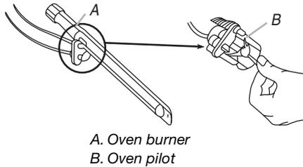
6. Hold the oven control knob in for 10 seconds to make sure the pilot will remain lit.
