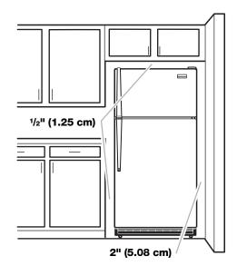
To ensure proper ventilation for your refrigerator, allow for a %" (1.25 cm) space on each side and at the top. Allow at least 1" (2.54 cm) between back of cabinet and the wall. If your refrigerator has an ice maker, make sure you leave some extra space at the back for the water line connections.
