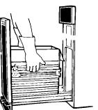
Lift the front to clear the drawer stops. Grasp the drawer on the sides.
