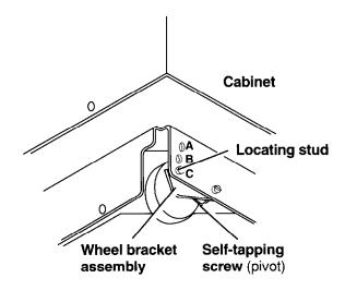
5. The rear wheels are preset for a cabinet opening height of 86.4 cm (Position "A"). To adjust for other heights, loosen screw just enough to clear stud from hole in Position "A." Move the rear wheel and stud to Position "B" or "C" as needed.
