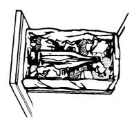
Bottles or cans not placed in the center may become caught between the ram and the drawer. The Drawer Monitor Switch senses a "misload" and causes the ram to return to the "up" position without compacting. Load bulky trash, bottles and cans in the **center** of the drawer.
