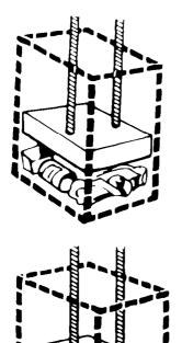
The compacting ram does not go to the drawer bottom. You will not see compacting of the first few loadings.
