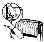
Push side-lock lever down and tilt drawer side open.
