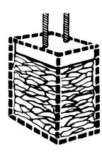
The trash in a full compactor bag will be about 1/4 the size of its original bulk.
