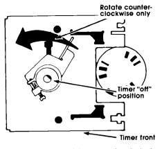
Coin-operated timers can be started by turning the clutch assembly counter-clockwise until the washer starts to fill with water.
