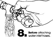
run water through both faucets into a bucket to get rid of particles in water lines.
