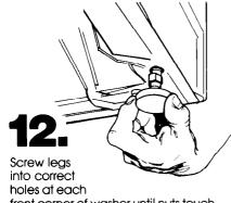
front corner of washer until nuts touch washer. **Do not** tighten nuts until step 15.
