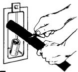
Move washer close to final position. Put "hook" end of drain hose into standpipe. Estimate length of drain hose needed when washer is in final position. Hose must be cut exactly to length so "hook"
