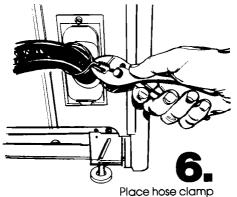
over washer drain connector. Push drain hose onto
