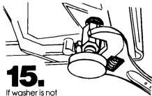
level, screw the front leas up or down to adjust. Make final check with level
