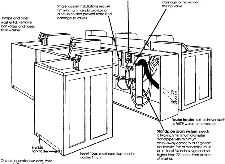
On coin-operated washers, front access to the pump area is available by removing the two No. 10 Torx screws and then removing the front panel. Non-coin operated washers do not have a removable front panel. The cabinet and top assembly must be removed by removing clips under console on the non-coin operated washer.
