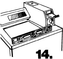
Tilt washer forward raising back legs 1" off of floor. Gently lower washer to floor. Check levelness at the washer front and from front to back on each side using a carpenter's level.
