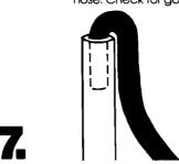
Put "hook" end of drain hose back into standpipe. Allow space between the standpipe and drain hose for an air gap. Too tight of a fit could cause siphoning.
