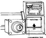
Put the coin vault with lock and key in the meter case opening. A larger capacity coin vault can be installed. Use a knife to carefully remove the paint along the seam at the bottom of the conversion bar. Use a blade screwdriver and a hammer to lightly tap along the seam area. Raise the conversion bar up to the notches in the sides of the vault opening. Remove the conversion bar and drawer guide. Install new guide (found in parts bag) and the larger coin vault.
