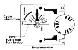
Non-coin operated timer cycle information is ink stamped on the rear of the timer. Push in on the lever attached to the timer shaft. Reset lever to the Normal cycle position then pull out on lever to start washer.
