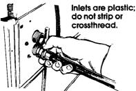
Attach hose to bottom inlet valve opening first. Then second hose to top inlet. Tighten couplings by hand; then use pliers to make an additional two-thirds turn,
