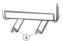
Stack two corner posts (A) on top of each other. Tilt washer backwards and slide corner posts under washer 7.6 cm (3 inches) from each side of washer as shown.
