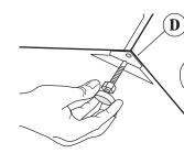
Insert legs into correct holes at each front corner of washer until nuts touch washer (**D**). **DO NOT** tighten nuts until washer is level.
