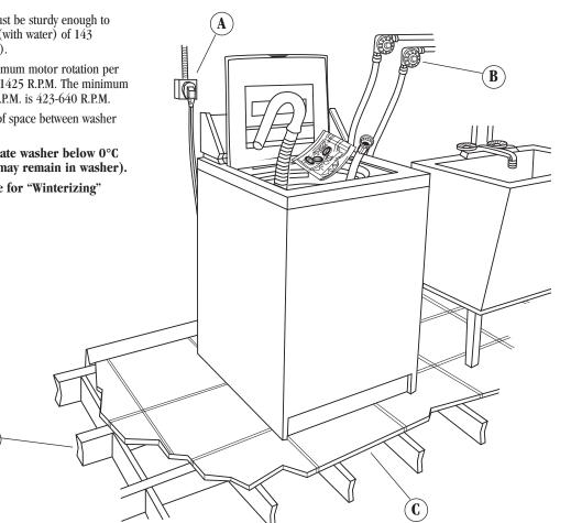
The installation dimensions shown are the minimum spaces allowable. Additional spacing should be considered for ease of installation and servicing.
