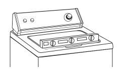
Tilt washer forward, raising back legs 2.5 cm (1 inch) off of floor to adjust rear self-leveling legs. Drop washer to floor. Check levelness of the washer by placing a carpenter's level on top of the washer, first side to side; then front to back.
