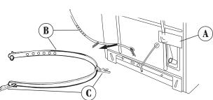
SLIDE WASHER ONTO CARDBOARD OR HARDBOARD BEFORE MOVING ACROSS FLOOR.
