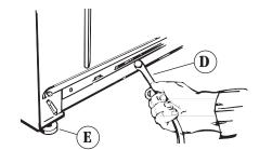
Pull firmly to remove the other end of the shipping strap (D) from the back of the washer to release self-leveling legs (E).
