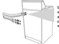
Check inlet hoses periodically. Replace inlet hoses if you find bulges, kinks, cuts, wear or leaking. Replace inlet
