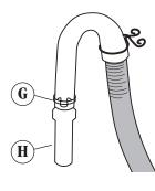
If drain hose does not fit into standpipe or is being placed over the edge of a laundry tub, open other drain hose clamp with pliers and place clamp over rubber end of drain hose (G).
