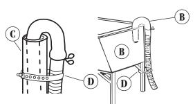
Check that hose is not twisted or kinked and is securely in place.
