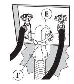
If the water inlet faucets and drain standpipe are recessed, put "hook" end of drain hose (E) in standpipe. Tightly wrap the shipping strap (F) around the drain hose and faucet body (not the handle or stem). Push plug into the nearest hole in the shipping strap.
