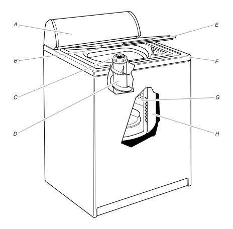
A. Control panel B. Model and serial number label C. Liquid fabric softener dispenser D. Agitator
