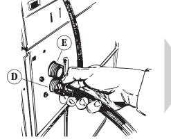
Attach hose to hot water (bottom) inlet valve (**D**) first; then second hose to cold water (top) inlet valve (**E**). Tighten couplings by hand. Then use pliers to make additional two thirds turn.
