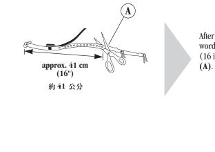
After shipping strap has been removed from washer, look for the words "cut here" marked on the shipping strap, about 41 cm (16 inches) from the plug end. Cut the shipping strap at this mark **(A)**.
