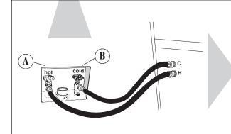
Attach bottom hose from the inlet marked "H" to hot water faucet (A). Attach top hose from the inlet marked "C" to cold water faucet (B). Tighten couplings to faucets by hand; then use pliers to make additional two-thirds turn. **Do Not overtighten;** this could cause damage to couplings.
