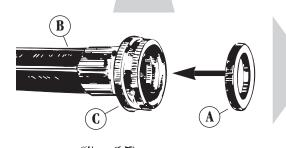
Insert a flat washer (A) into **each** end of the inlet hoses (B). Check that washers are firmly seated in couplings (C).
