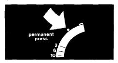
There is a dot just after the numbers in PERMANENT PRESS, REGULAR HEAVY and KNITS GENTLE. If you push in on the Cycle Control Knob, turn the pointer to one of those dots and pull the Control Knob out, the washer will fill, agitate, drain and spin
