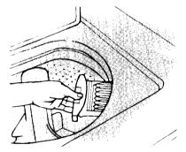
Water runs through the lint filter whenever the washer agitates. Check it often to make sure it's clean and filtering at its best.
