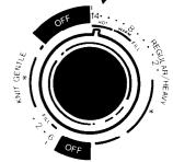
• Hot wash can be selected only in the REGULAR HEAVY Cycle. Push in and turn the Cycle Control Knob so the pointer is on from 10 to 14 minutes in the REGULAR HEAVY Cycle. Pull the Control Knob out to start.
