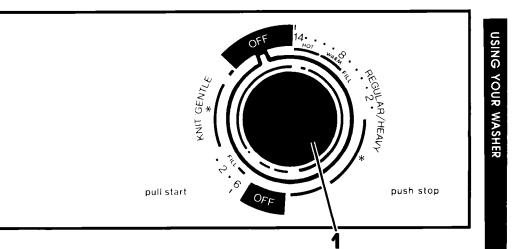
A warm wash is pre-set in the KNIT GENTLE Cycle. Push in and turn the Control Knob so the pointer is on from 4 to 6 minutes. Pull the Control Knob out to start.
