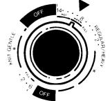
• Warm wash can be selected in the REGULAR HEAVY Cycle. Push in and turn the Cycle Control Knob so the pointer is on from 7 to 9 minutes. Pull the Control Knob out to start.
