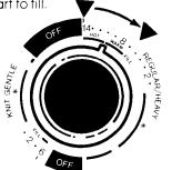
• When there is as much water as you want in the washer, push the Control Knob in. **SLOWLY** turn it to the right, past the fill area. Pull the Control Knob
