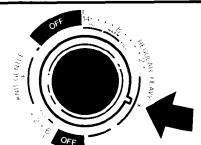
temperature in the REGULAR HEAVY Cycle. You can also work the Cycle Control Knob to use less water when washing small loads. (See page 5.) If you turn to a cycle and start the washer, but change your mind, push in on the Cycle Control Knob and turn to the right (clockwise) to the setting you want. Then pull out to start.
