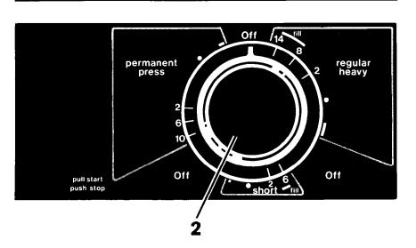
• To use less water, push the Controi Knob in and turn to the right (clockwise) to a fill area in either the REGULAR HEAVY or SHORT Cycle. (PERMANENT PRESS fills to the highest level.)
