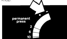
To set the washer so it drains and spins water out of the load, push in on the Control Knob, turn the dial to the right (clockwise) so the pointer is touching the bar just before OFF in any cycle.
