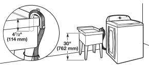
Minimum capacity: 20 gal. (76 L). Top of laundry tub must be at least 39" (990 mm) above floor; install no higher than 96" (2.44 m) from bottom of washer.
