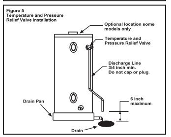
For protection against excessive pressures and temperatures, a temperature and pressure relief valve must be installed in the opening marked "T & P RELIEF VALVE" (See Figure 5).
