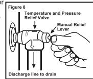
temperature and pressure relief valve to allow the valve to operate freely and return to its closed position. If the valve fails to completely reset and continues to release water, immediately shut off the electrical power and the cold water inlet valve and call a qualified service technician.
