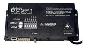
The DCSP1 is a regulated low-noise 48VDC power supply that can deliver up to 500mA. (Approximately 48 channels of microphones at 10mA each.)
