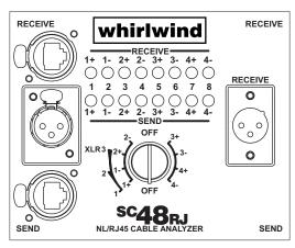
The Whirlwind SC48RJ Cable Analyzer is a convenient device for fully testing professional NL multiline speaker cables, RJ45 Ethernet cables and three pin XLR cables. The simple yet comprehensive design can diagnose opens, shorts, incorrect wiring or even customized wiring configurations in cables with up to eight conductors. The SC48 is powered by a single 9 Volt battery.
