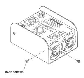
Removing the six case screws provides access to the 9 Volt battery compartment. The battery should be changed when the SEND LED becomes dim.
