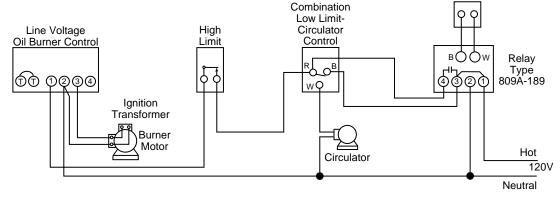
The low limit side of the low limit/circulator control maintains domestic hot water temperature all year around. When the room thermostat calls for heat, the burner and
