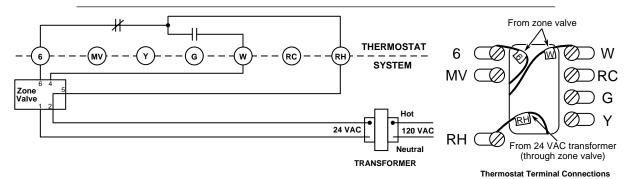
Figure 10. Typical wiring diagram for heat only, 3-wire, zone valve systems
