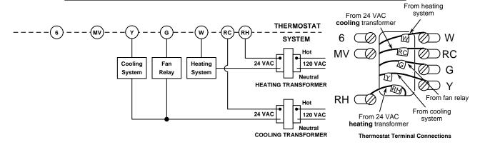
Figure 11. Typical wiring diagram for heat/cool, 5-wire, two-transformer system
