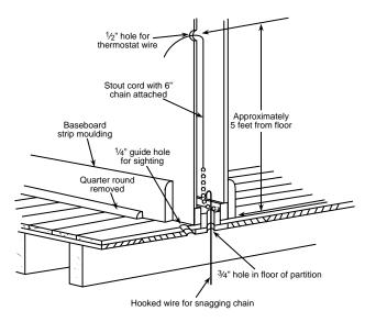
Figure 1. Routing thermostat wires
