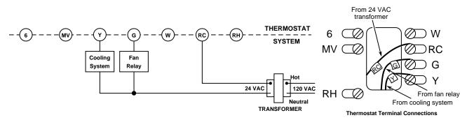
Figure 6. Typical wiring diagram for cool only, 3-wire, single transformer systems
