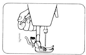
When you fail to catch the foot, push the lever in the arrow direction slightly.
