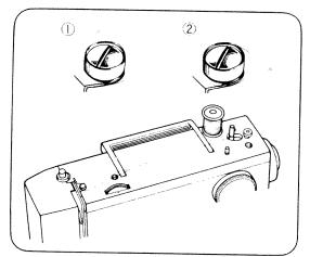
Wind thread clockwise around bobbin several times. Push bobbin on to spindle.
