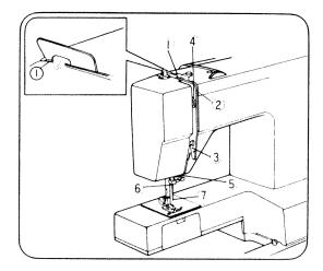
Lead thread either side of tension disc (2).
