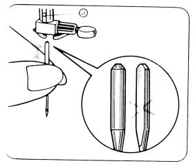
With flat face away from you, insert a new needle into groove of needle bar.
