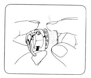
Guide thread into slot (a) of bobbin case.
