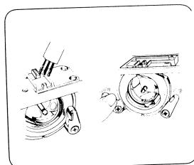
Remove shuttle race cover. Remove shuttle Clean shuttle race with a cleaning brush and a soft cloth.
