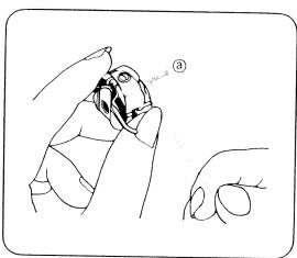
Pulling thread to left, bring it under tension spring then to delivery eye **b**.
