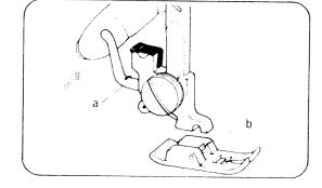
Lower the presser foot lifter so that the foot will be automatically snapped on.
