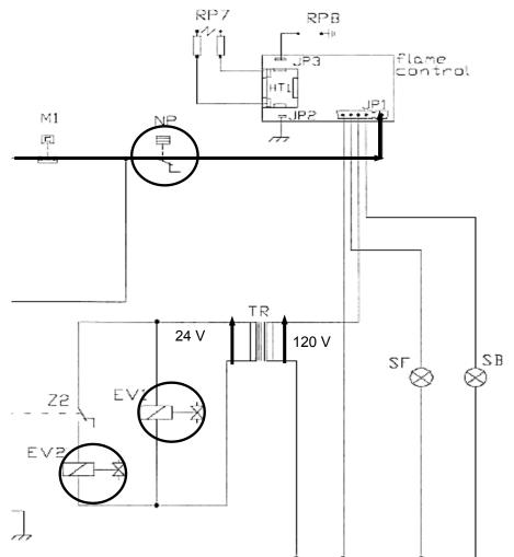
Point 13 (TR) No inlet voltage (120 V). Check 5 pole connector and control box. If everything is okay, replace the connector.
