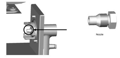
3. Change the nozzle, attach the screw indicated at point 1 and set the burner pressure as indicated in the table below:
