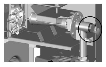
2. Without removing anything else, remove the nozzle from the burner inserting the screwdriver as indicated by the arrow.
