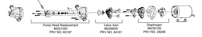
PUMP REPLACEMENT PARTS FOR FLOJET 100 PSI (86251110 - PRV NO. 65219)
