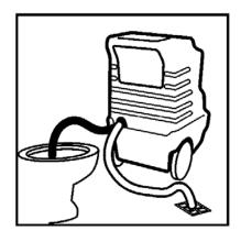
11. Drain machine at proper disposal areas. Use pressure gun to rinse and clean recovery tank.
