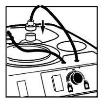
Attach the adapter cap and intake hose to the Compass<sub>™</sub> Chemical bottle. Refer to the Compass<sub>™</sub> Chemical Label for the desired dilution.
