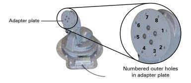
Note: as the antenna raises and turns, the adapter plate may become skewed, and the fourth hole may not be directly at the bottom of the plate. If unsure of the fourth hole, remove the four screws from the center of the adapter plate; a small post is located directly above the fourth hole.
