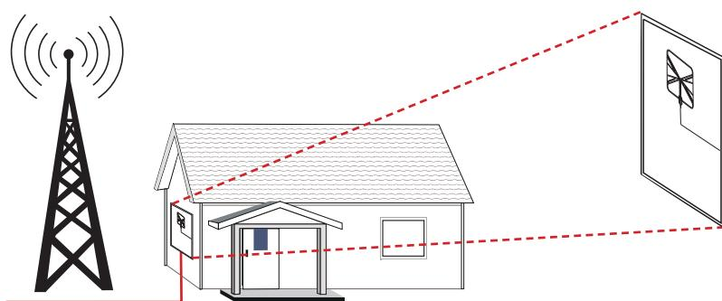
If the antenna is mounted so that it hangs vertically, the coax cable should run from the top or bottom of the antenna. If the antenna is mounted so that it lies flat (e.g. on a table), the coax cable should point toward the signal.
