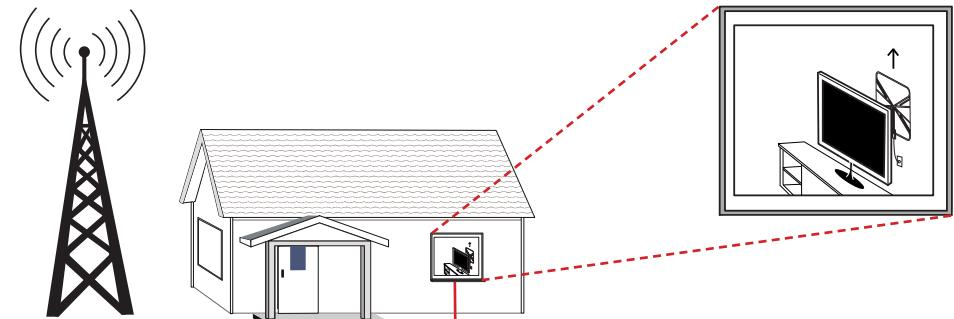
The antenna may pick up signal when mounted near electronics, or electronics, including the television itself, may reflect the signal from the broadcast tower. If so, try mounting the antenna higher on the wall, and run a new channel scan. The higher the antenna, the better signal you will receive.
