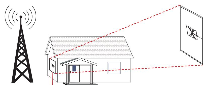
The coax cable is running from the side of the antenna instead of the top or bottom of the antenna. Try re-positioning the antenna so that the coax cable runs from the top or bottom of the antenna, and run a new channel scan.
