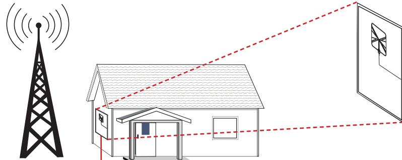
Mount the antenna on a window that faces the broadcast tower or stations that you want to receive. The sides of the antenna have blind spots, so the antenna may not "see" enough signal from the broadcast tower if the sides of the antenna face the tower.
