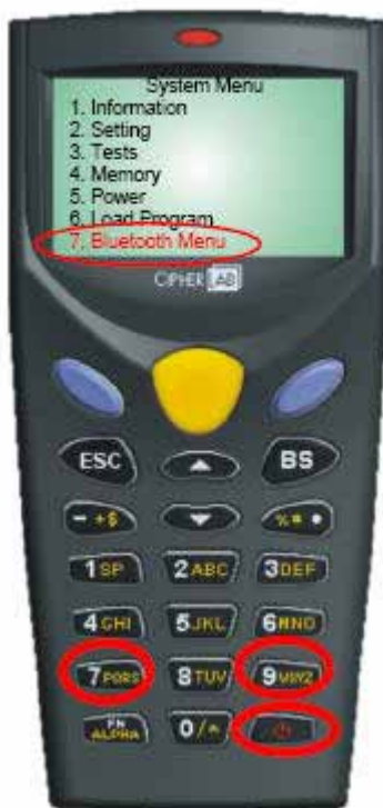
Figure 69: Accessing Wireless Scanner Main Menu Simultaneously Press <7> + <9> + <Power>, When in System Menu, press <7>, followed by <Blue Enter>
