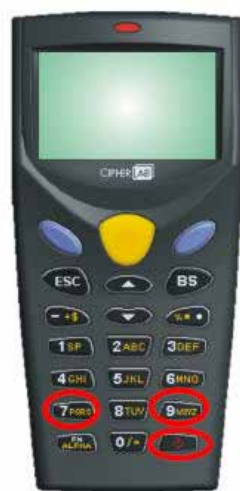
Figure 81: Powering the Scanner On and Off Simultaneously Press <7> + <9> + <Power>, After three beeps, turn scanner off by pressing <Power> again
